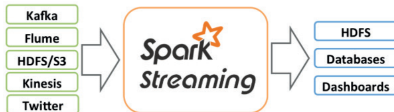
Figura 4. Spark Streaming Data Sources. Obtenido de: https://spark.apache.org/docs/latest/streaming-programming-guide.html
